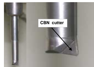
Fig. 2. CBN end mill applied in the research
